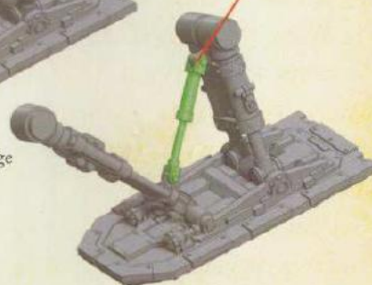
35. Rear Undercarriage Retraction Actuator
