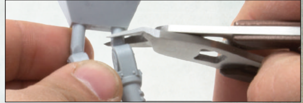
Clippers being used to remove the casting gates.
