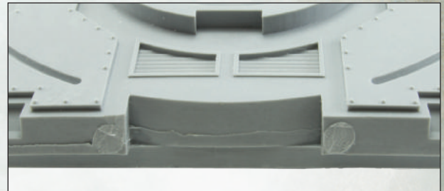
This component has a mould line and some excess resin resulting from the casting gate removal process.
