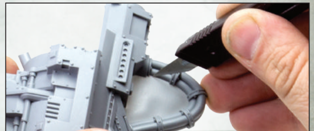
Shims are easily removed by cutting their edges with a modelling knife.
