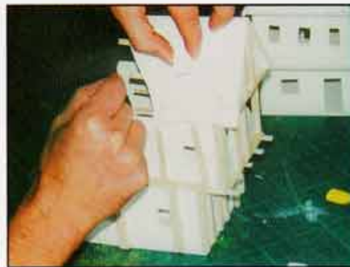
Using strips of balsa wood (or strips cut from foamboard), create extra detailing on the exterior of the building.
