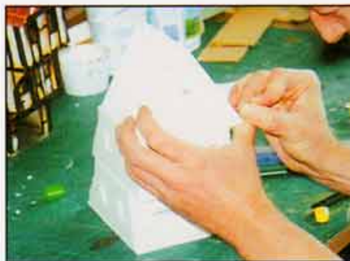
Finish the basic structure with the addition of the roof, made from three pieces of foamboard with a window cut into the triangular front facing.
